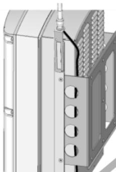
Figure 3: Routing the antenna cable (three phase inverter)
