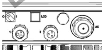
Figure 4: Inverter sealing glands
