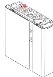
① For the new version battery, there is no need to remove the top cover in Step 3.
